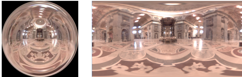
Figure 4.7: Light probe image captured at St. Peter’s Basilica in Rome. The left image shows the original light probe image, and the right image shows a latitude-longitude projection of the same environment.
